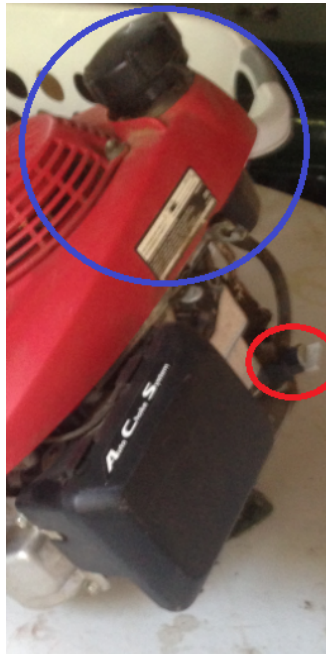
Figure 16-Fuel tank (blue) is molded into flywheel cover, and gravity feeds through a shutoff valve (red) to the carburetor
