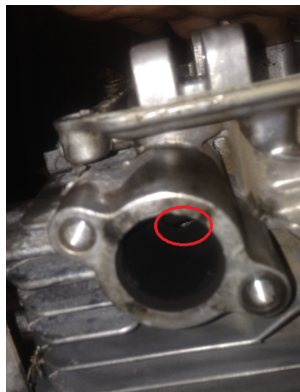
Figure 13- Exhaust path is cast directly into block. Circled in red is exhaust valve port.
