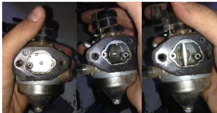
Figure 7- Left to Right, choke plate positions are actuated from fully closed to fully open via the choke control arm
