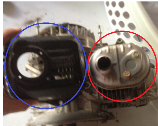
Figure 14-Heat guard (blue) covers muffler (red) during normal operation
