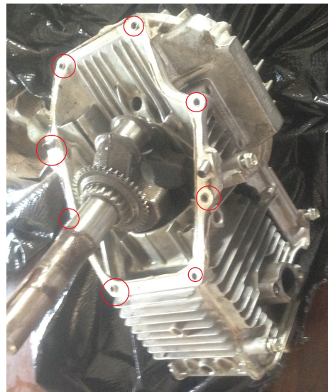
Figure 2- Locations of 8 #10 bolts used to secure crankcase to block
