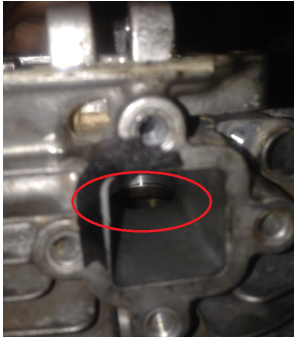
Figure 11-Intake path is cast directly into block. Circled in red is intake valve port.
