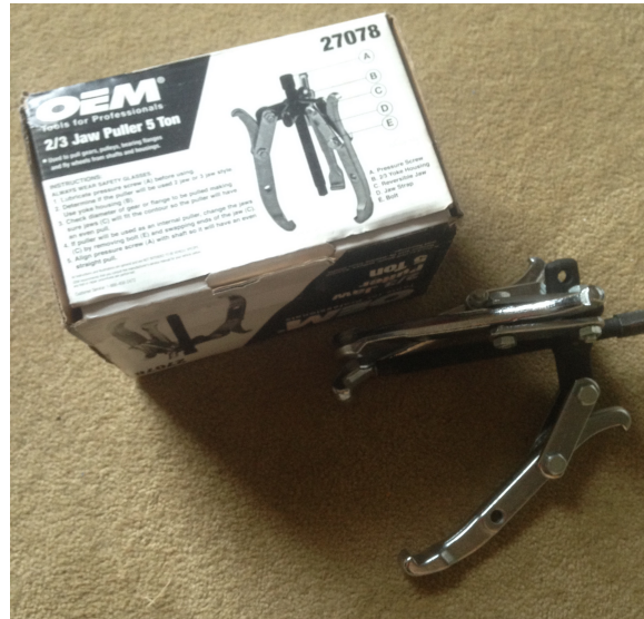
Figure 1-Free Rental Flywheel Puller Made Removal of Flywheel Much Easier
