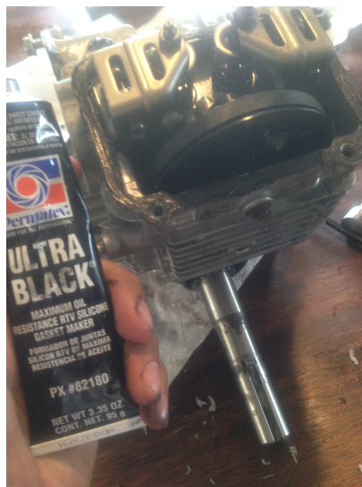
Figure 5- Silicon gasket maker was used to seal valve cover and crankcase
