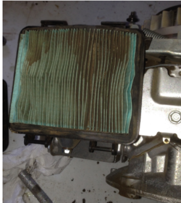
Figure 10- Air enters engine through a paper filter in the air box
