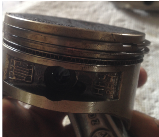
Figure 20- Piston with rings installed
