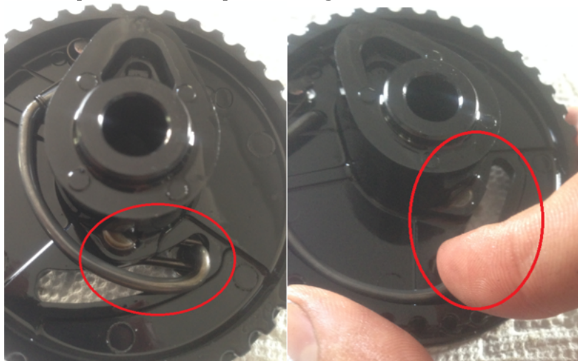
Figure 9- Cam gear in low RPM mode has lobe present (left), at high RPM the lobe is rotated to a flat shape (right)
